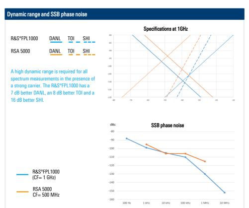
A low phase noise is required for spectral measurements close to the carrier. The R&S\*FPL1000 outperforms the RSA5000 by up to 20 dB. RIGOL specifies the SSB phase noise at a CF of 500 MHz (R&S\*FPL: 1 GHz), leading to better SSB PN values of the RSA5000 (a few dB in this comparison). The RSA5000 also seems to be optimized for an offset of 10 kHz.
