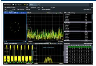
Analysis of a Bluetooth 3-DH1 signal. Constellation diagram, EVM, result summary, magnitude, spectrum and symbols with pattern detection all in one view.
