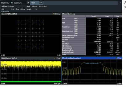
Analysis of a 640AM signal with the R&S®FPL1-K70 vector signal analysis option
