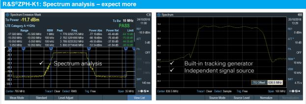
R&S°ZPH-K1 enables spectrum analysis and features an integrated tracking generator and an independent signal source. As the signal source, the R&S°ZPH-K1 can generate a CW signal at any frequency, or the R&S°ZPH-K1 can be coupled to the center frequency. This feature is useful for frequency conversion measurements.
