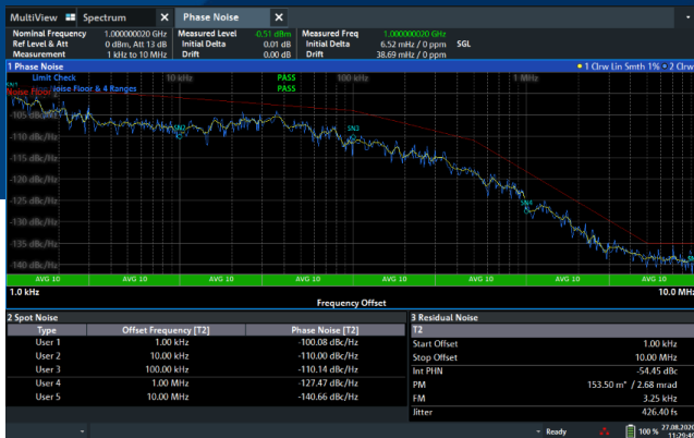
Phase noise measurement plus automatic limit checking, spot noise and residual noise indication.
