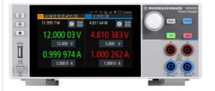
When the power supply is in constant voltage mode, the numbers and the keys are green. Red is used for constant current mode. The output key lights up blue to indicate that the channels are switched on (active).
