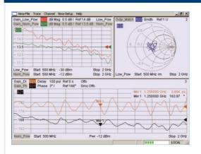
Several traces can be combined in diagrams and assigned to different measurement channels.
