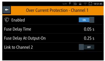
The user can set safety limits to restrict the adjustment range of the power supply and prevent a DUT from being damaged due to accidentally using the wrong setting.
