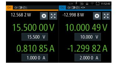
The measured currents and voltages are displayed with 6 ½ digit resolution. The
