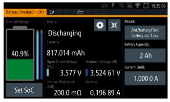
The battery simulation software includes data sets of common battery types that can be modified easily.
