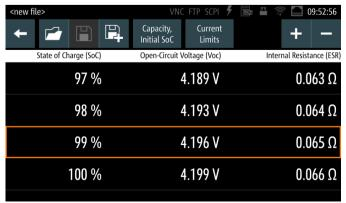
Battery simulation can be performed simultaneously on both channels with the twochannel R&S®NGM202.
