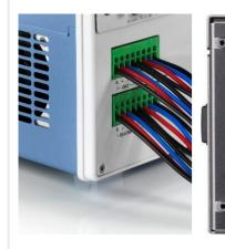
Connections for all channels - including sense lines - are also provided on the rear panel (R&S and Keysight)
