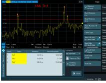
The R&S°ZNL-K3 option lets the analyzer automatically determine a suitable number of sweep points for a given maximum distance to fault. It is also possible
