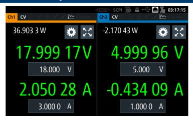
A resolution of up to 6½ digits is perfect for characterizing DUTs that have low power consumption in standby mode and high current in full load operation. The R&S\*NGM200 power supplies automatically switch between source and sink mode. A negative current reading indicates that the instrument operates as a load.
