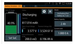
Capacity, open circuit voltage (Voc) and equivalent series resistance (ESR) are important battery characteristics that are based on the battery's state of charge (SoC). The optional R&S®NGM-K106 battery simulator allows users to simulate battery behavior under different charging conditions, such as when powering a DUT.
