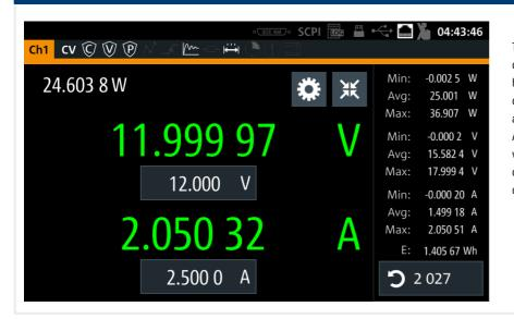
The large capacitive touchscreen is the central operating element. With its very high resolution of 800 x 480 pixel, the display makes it easy to read the voltage and current fields even at great distances. Additionally, information such as power values or statistics can be displayed. Icons clearly show the status of the set protection or special functions.
