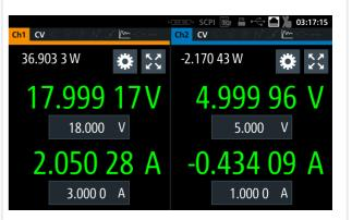
A resolution of up to 6 ½ digits is perfect for characterizing DUTs that have low power consumption in standby mode and high current in full load operation. The R&S®NGL200 power supplies automatically switch from source to sink mode. Operating as a load is indicated by a negative current reading.
