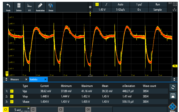
Power integrity measurement
