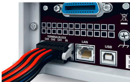
WAGO cage clamp: To facilitate typical calibration setups, the rear panel connector was designed with a WAGO cage clamp.
