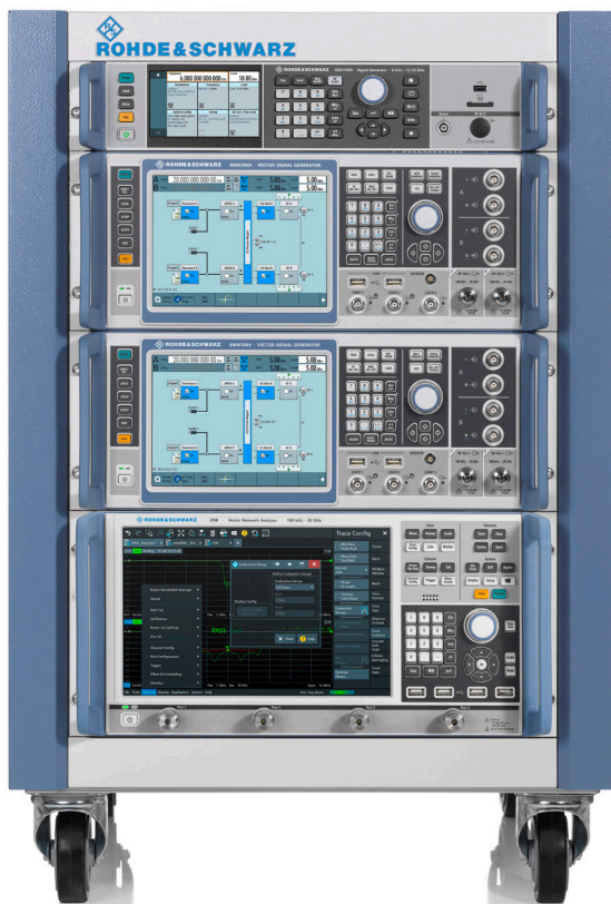
Four-channel radar test system consisting of two R&S®SMW200A vector signal generators, an analog R&S®SMA100B signal generator providing the LO signal and a Rohde & Schwarz vector network analyzer for the automated RF port alignment.
