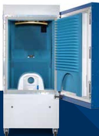
The compact R&S®ATS1800C mmWave chamber.
