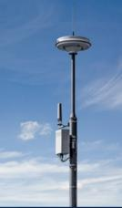
Rohde & Schwarz spectrum monitoring systems can be configured for automatic measurements and run autonomously. The portfolio's efficient solutions comprise various fixed, transportable and portable spectrum monitoring stations for various applications. The systems provide extensive spectrum awareness within and around specific areas and facilities.
