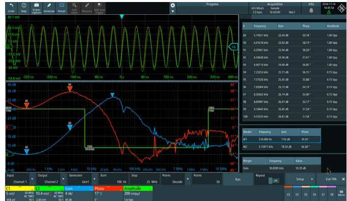
PSRR measurement using R&S®MXO-K36 frequency response analysis software option
