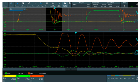
The MXO digital trigger is useful when analyzing the scenario and helps make sure designs have enough dead-time between the switching of high-side and low-side gates.
