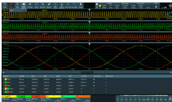
MXO with track function can visualize PWM into traces for analysis
