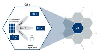
privacy protection or target localization through accurate object location finding alongside the establishment of communications links. A new waveform must be designed for ISAC. Starting with coordinated signals where a radarcentric or a communication-centric development approach is possible, the true goal is a fully unified waveform that integrates both radar sensing and communications for the best possible solution.
