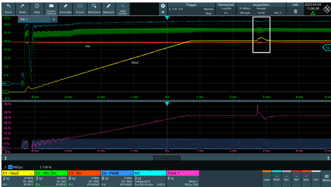
Fig. 5: Startup of the converter and irregular control effects
