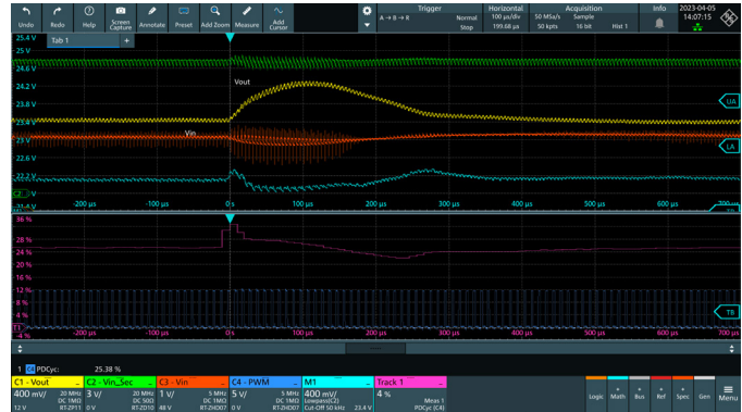
Fig. 6: Irregular control effects at trigger condition B
