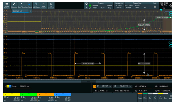
Fig. 3: PWM details in steady state of the converter
