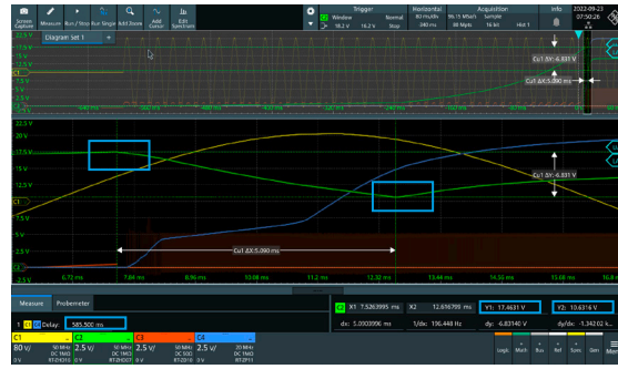
Fig. 2: Startup sequence measurement of the converter
