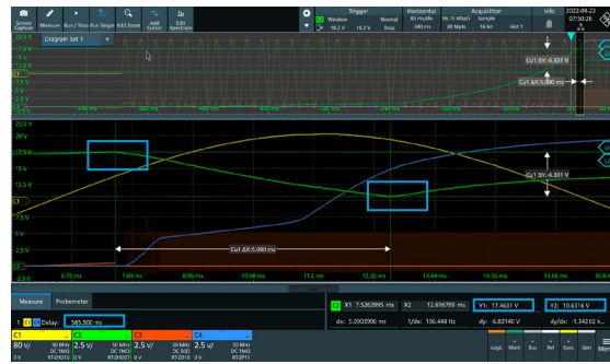
Fig. 2: Startup sequence measurement of the converter
