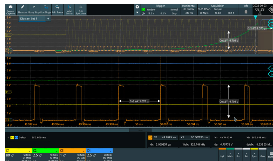
Fig. 3: PWM details in steady state of the converter
