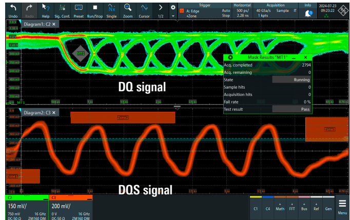
Mask test applied to a continuously running WRITE acquisition. On the DQ signal, a color table is applied to visualize the statistical distribution of the DQ data signal.
