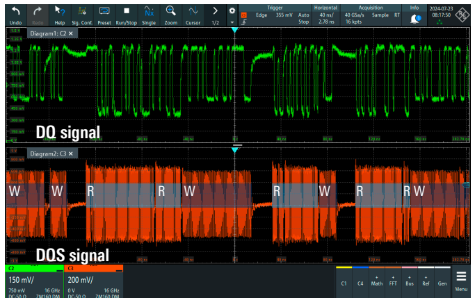
DDR4 DQ (C2: green) and DQS (C3: orange) signals with READ and WRITE bursts. In this example, a visual distinction between READ/WRITE bursts is possible based on the amplitude. (R: READ; W: WRITE)
