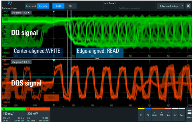
Zone 1 with excluded intersect on DQS signal focuses acquisition to start of READ and WRITE bursts with no activity happening before.
