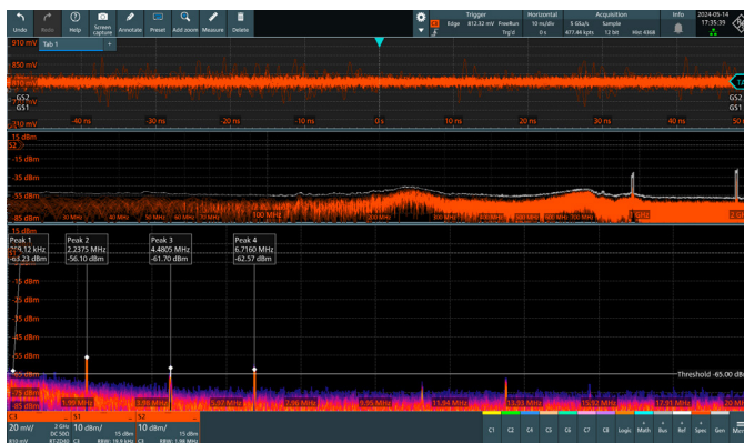
Power integrity analysis in time and frequency domain, showing the 2.24 MHz switching frequency and its harmonics
