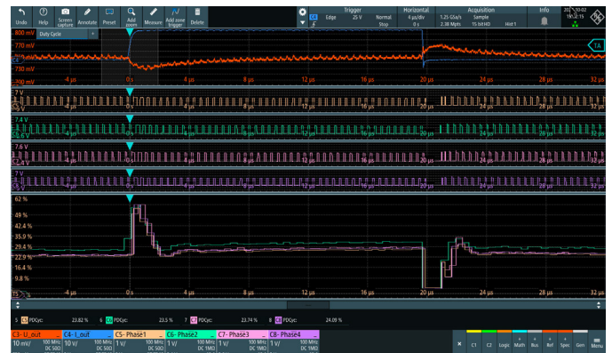
Phase alignment and PWM track in a dynamic load step scenario, continuously turning on/off a 160 A load. Waveform and PWM track show an immediate reaction of the phases on the load steps.
