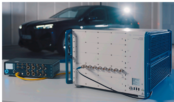
eCall speech quality test setup
