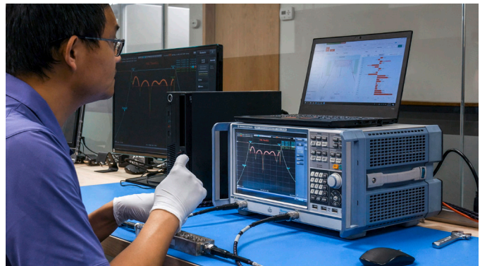
Rohde & Schwarz and SynMatrix tuning solution setup
