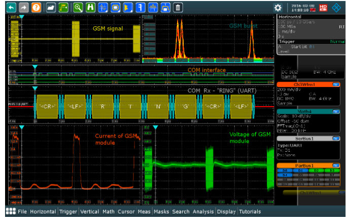
GSM connection of an IoT module.
