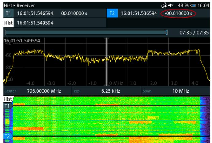
Fig. 8: Measuring the periodicity of suspected broadcast bursts (red circle)
