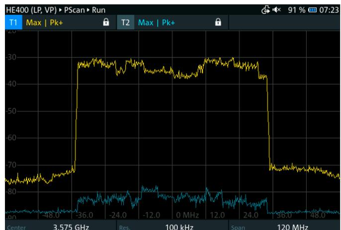
Fig. 14: Estimation of unwanted sideband emissions during traffic
