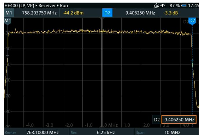
Fig. 4: Bandwidth and center frequency measurement of signals narrower than 40 MHz
