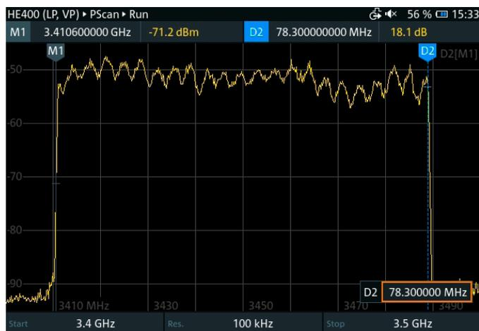
Fig. 5: Bandwidth and center frequency measurement of signals wider than 40 MHz
