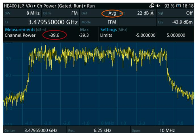
Fig. 16: Measurement of the SSB channel power (red circle) in persistent gated mode
