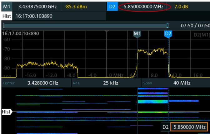
Fig. 9: Suspected 5G NR SSB, but with wrong bandwidth (red circle)
