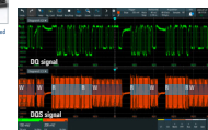
DDR4 DQ and DQS signals with READ and WRITE bursts. In this example, a read detection between READ/WRITE bursts is possible based on the analysis of RANCOM test mode.
