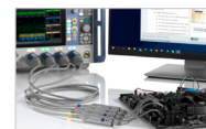
R&S®RTP high-performance oscilloscope with high-speed modular probes connected to the DDR memory interface for signal integrity debugging and verification
