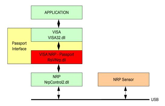
Note: Although the above picture illustrates only 32-bit modules the R&S®NRP VISA Passport driver is available in both 32-bit and 64-bit versions.
