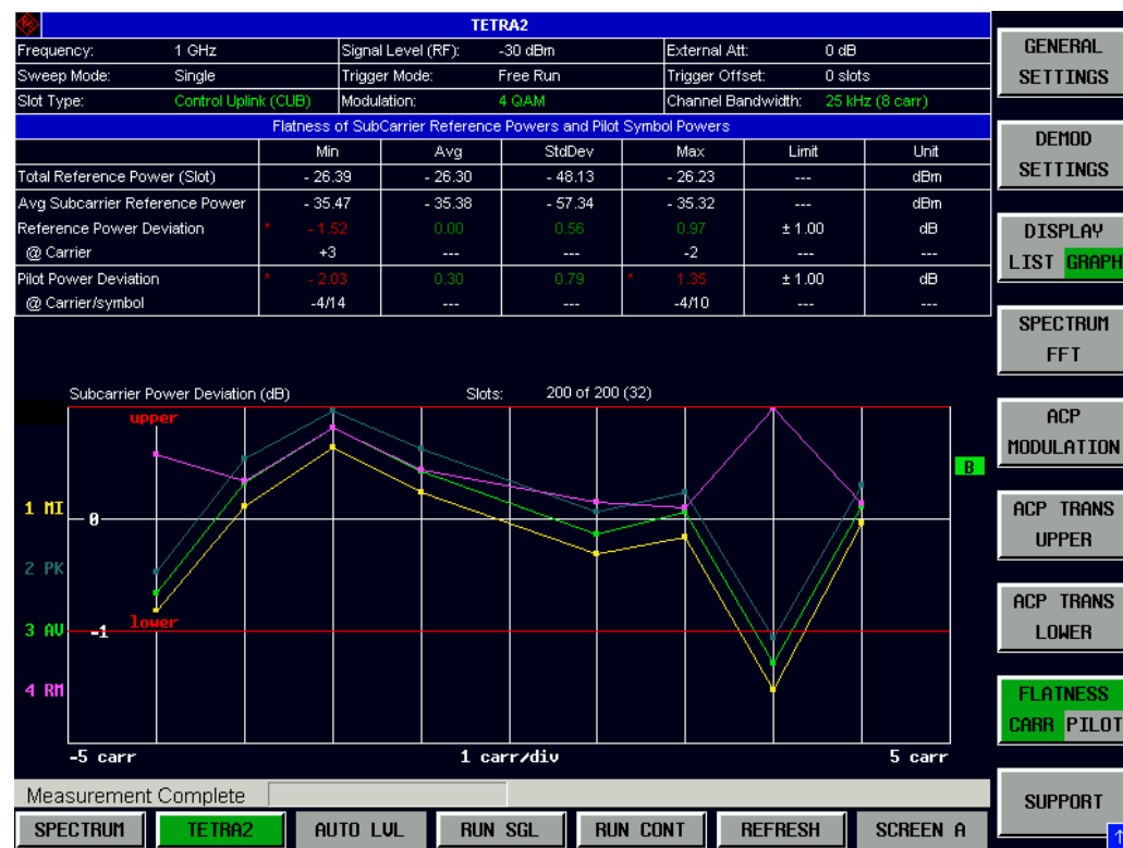
Fig. 23 Flatness measurement (example): Subcarrier Power Deviation
