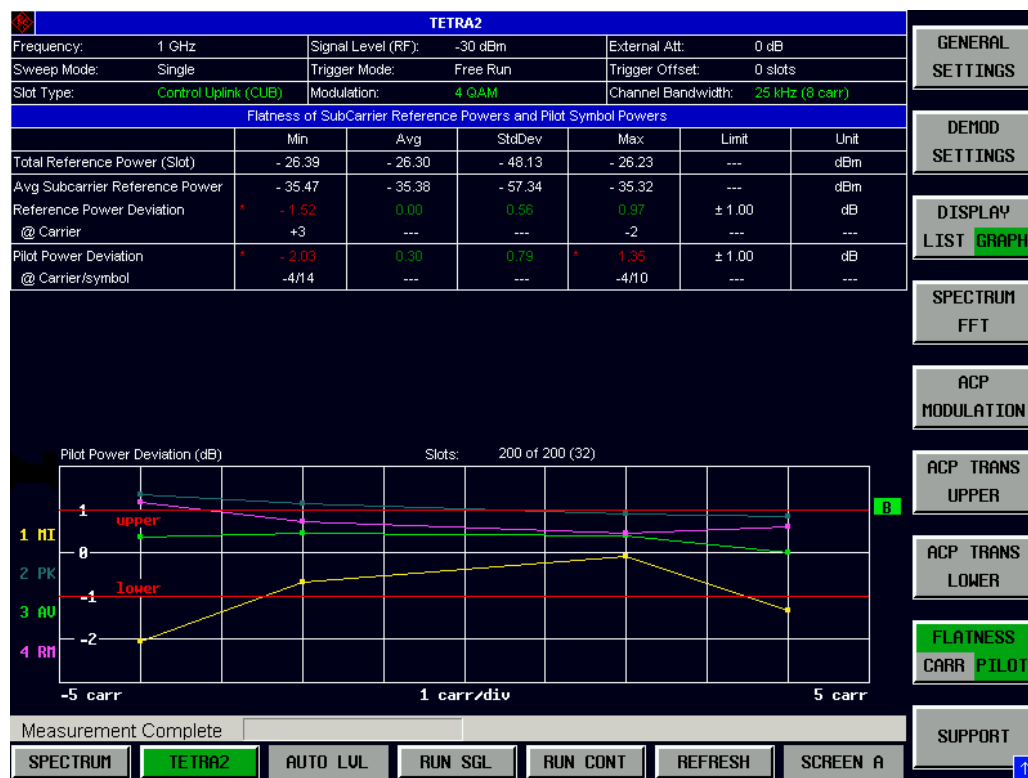
Fig. 24 Flatness measurement (example): Pilot Symbol Power Deviation
