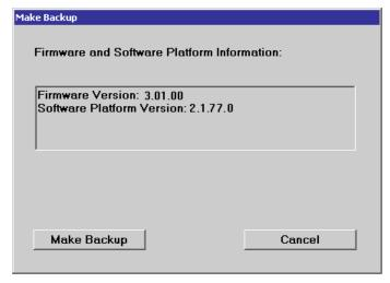
Select Make Backup and follow the instructions on the screenand the instrument starts working. The backup process takes some minutes. Please do not switch off the instrument, otherwise your backup may be corrupt. It's safe to switch off the instrument with the Exit and Shutdown button, when the menu is shown again.
