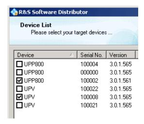
If no audio analyzers are found even if they are connected to GPIB or LAN, please ensure that the **Device Group** is set to "AUDIOANALYZER" and perform a rescan.
