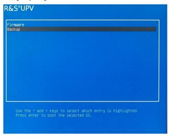
To manage the Backups you have to choose "Backup" with the direction keys within the 2 seconds. After a while following screen appears:
