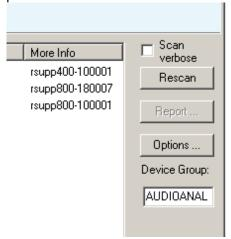
To store Device Group "AUDIOANALYZER" permanently, select "Options ..."-Button and type "AUDIOANALYZER" in the field shown below,
