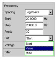
The new menu item **Halt** defines the frequency of the generator after the sweep has terminated.
