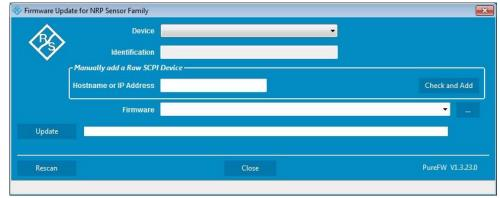
The program automatically starts scanning for R&S NRP-Zxx power sensors. When the scan is completed, all recognized power sensors are listed in the "Device" dropdown control.
