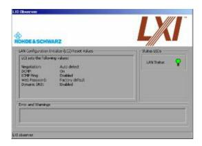
Pressing LCI will initiate the network configuration reset mechanism (LCI) for the instrument.
