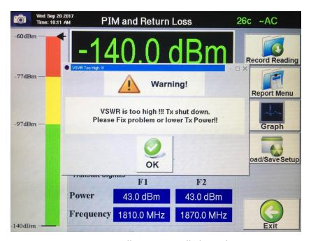
2) **TX Output Limit** – Unit will automatically limit the TX Output Power to a maximum of +43 dBm (20 Watts) when the PiMPro temperature reaches +50°C.
