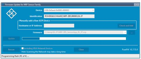
During the update process the progress is shown through a progress bar. The update sequence may take a couple of minutes, depending on the sensor model and the size of the selected file.
