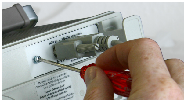
Fig. 2.1: Remove fastening screws
