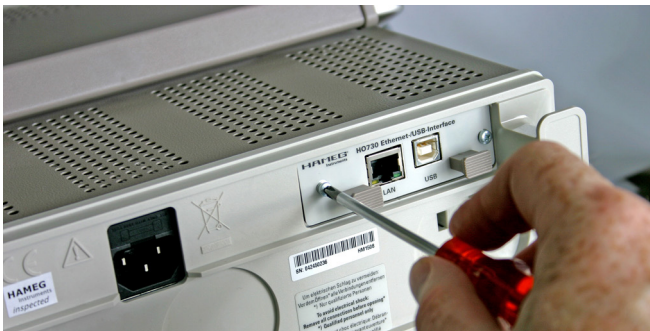
Fig. 2.4: Fastening screws
