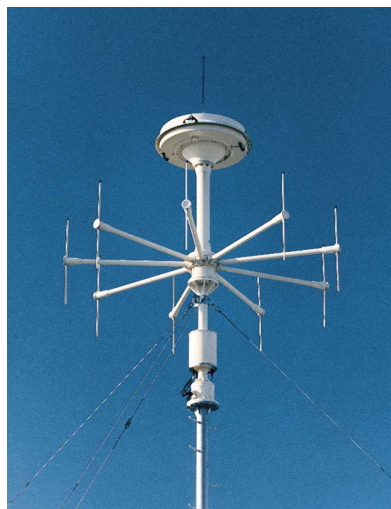
FIG 3 DF Antennas ADD051 and ADD070 for frequency range 20 to 3000 MHz
