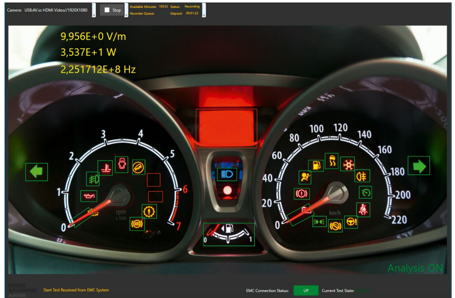
Fig. 2: Test view with superimposed information from an EMS test. All display elements are declared as ROIs and are monitored for changes.
