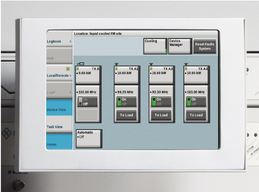
Fig. 3: R&S®TDU900 transmitter display unit showing a 3 + 1 system with 10 kW output power per transmitter.
