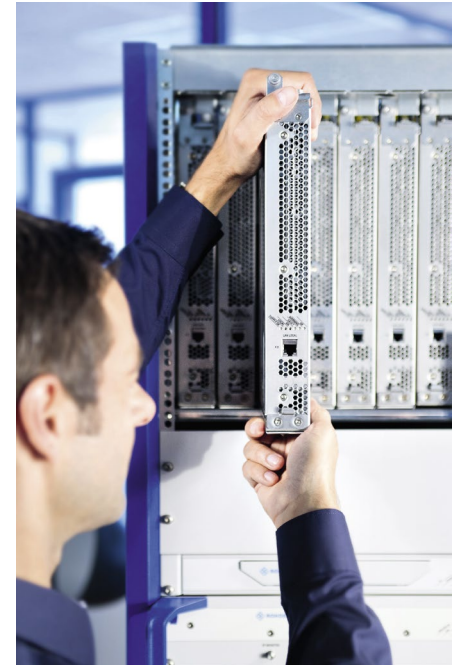
Fig. 4: The R&S®TCE900 exciter is configured with plug-ins and can be upgraded for HD Radio™.
