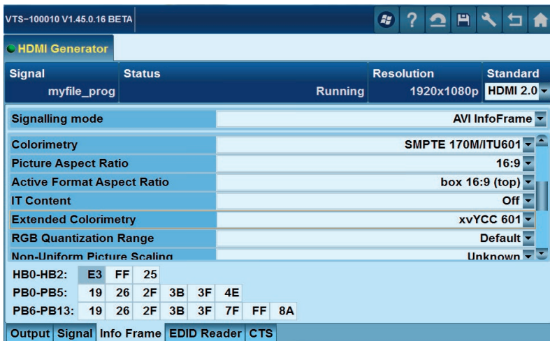
Fig. 3: The R&S®VT-K362 HDMI user defined option permits configuration of user-specific InfoFrame contents and other settings.
