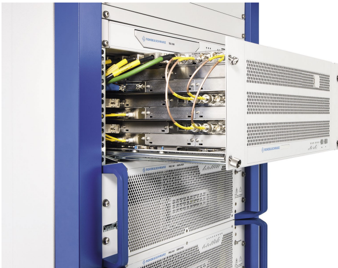
Fig. 2 The R&S®TMU9 can take on many different configurations: This picture shows R&S®TCE900 base units pulled from the rack. They can be configured either as exciters or as transmitter control units by changing the plug-in board.
