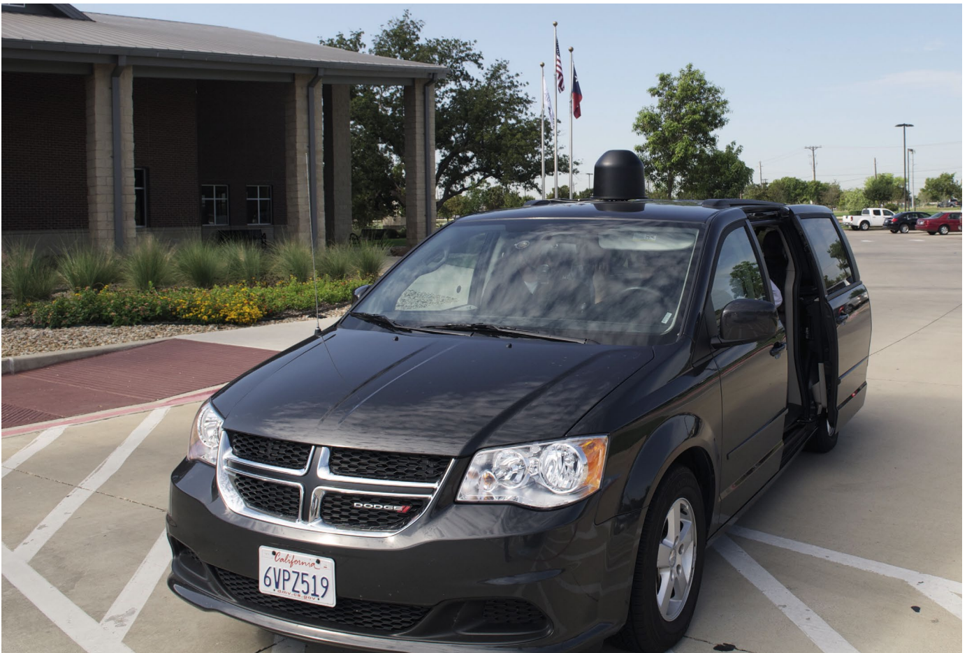
Fig. 4 DF vehicle with the R&S®ADD107 compact DF antenna (20 MHz to 1.3 GHz) and the R&S®DDF007 digital direction finder (in vehicle, not visible).
