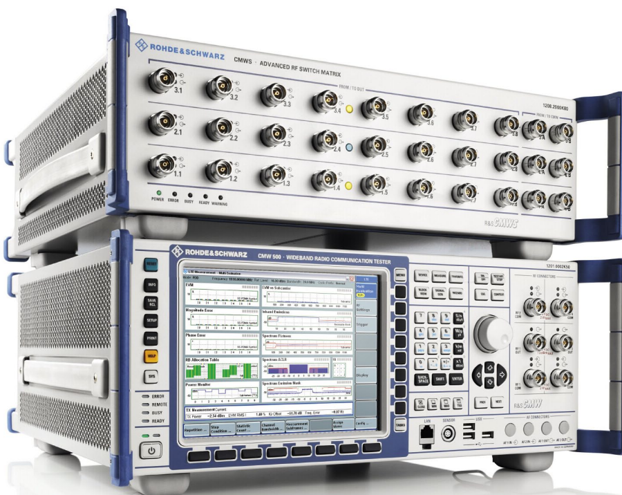
Fig. 1 Boosting efficiency in production: the R&S®CMW500 wideband radio communication tester with the R&S®CMWS advanced RF switch matrix. The R&S®CMWS simultaneously distributes the test signal from the R&S®CMW500 via its 24 RF ports to up to 24 DUTs.
