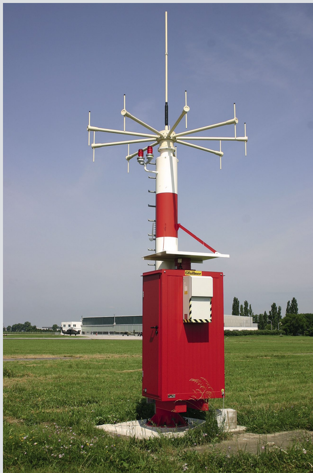
FIG 2 The R&S®DDF04E direction finder at Brumowski air base. An insulated and fully air-conditioned outdoor cabinet at the mast base houses the DF equipment and the DF server.
