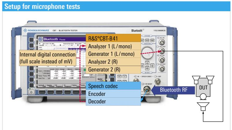
FIG 3 The two audio generators 1 and 2 independently generate test signals for the left-hand and the right-hand channels of the stereo signal. In this way, the two acoustic transducers in the stereo headphones are tested, as well as the analog components that are connected ahead.
