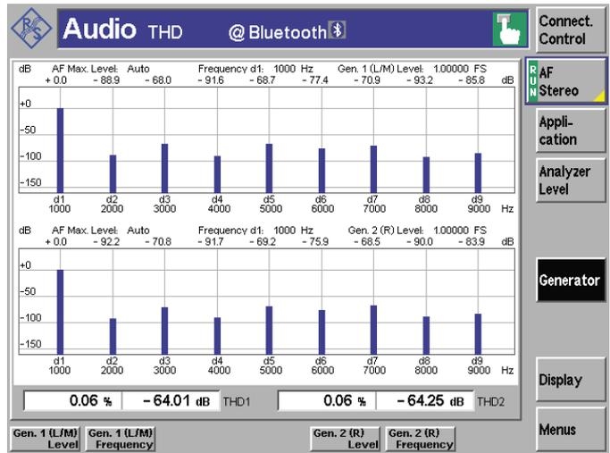
FIG 5 THD measurement of the two stereo channels.
