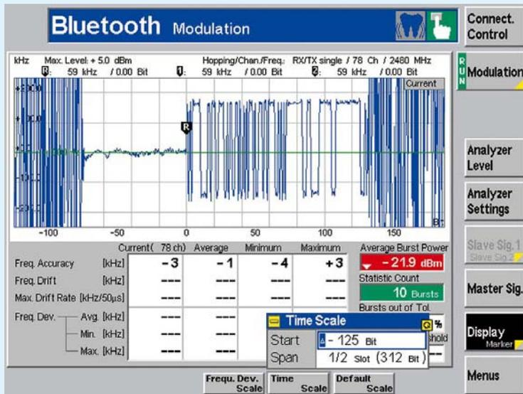
**FIG 7** Modulation measurement, stopped when limit exceeded.
