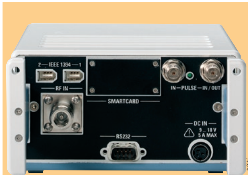
FIG 2 Rear view of the R&S®TSMU with synchronization and pulse input (top right), antenna socket and two FireWire connectors for cascading up to 62 R&S®TSMU analyzers on one controller. The RS-232-C interface supplies service information.
