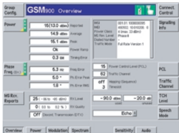
FIG 4 GSM Overview menu shows all important GSM parameters and results. Hotkeys (bottom) enable fast changing to special menus
